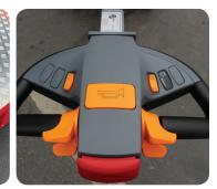
Drive backwards and forwards and the raise/lower function is controlled from the ergonomic control lever with built-in emergency stop.
