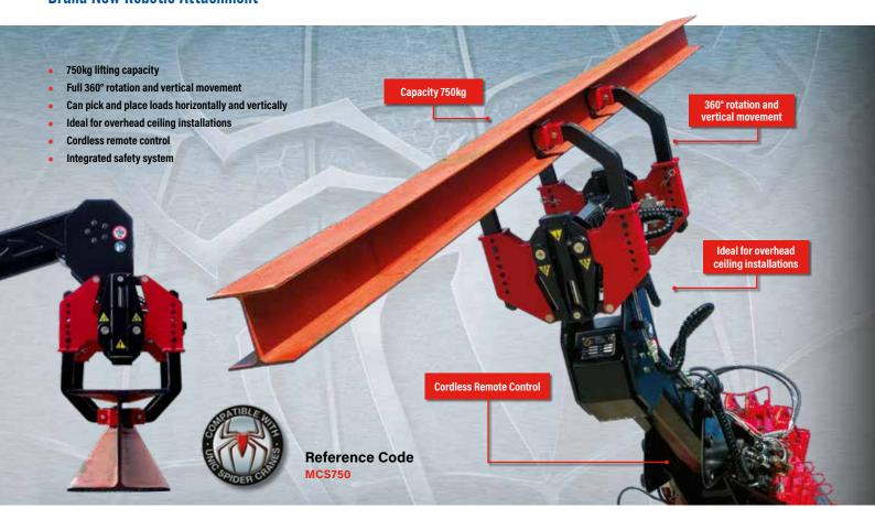
The MultiGrab is a hydraulic lifting clamp that has been designed for use with mini spider cranes and is able to lift to a capacity of 750kg. This innovative clamp is the perfect option for picking, rotating and placing steel,
