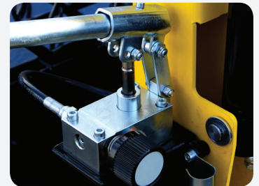
The boom of the Slewboy 500 is raised and lowered via a hydraulic pump and release wheel.
