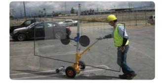
Extension arm available for lower glazing work and glass balustrading. Vacuum cups are 500mm (20") from the ground.
