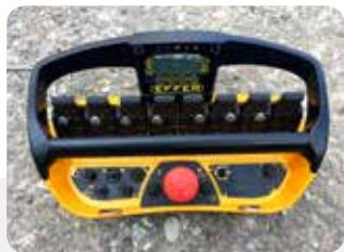
The TMC 525 radio remote control with digital feedback.
