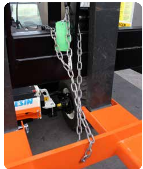
The Fork Mounted Hook comes with a safety retention chain that must always be used when attached to a forklift or telehandler.
