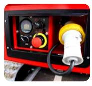
Simple on-board power switch controls and easy access charger makes using and recharging simple.
