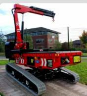
Able to pick up from the ground, lift loads onto it's own bed, track to the final location and install items over rough terrain makes the Tracked Leveller 5.5 with crane one of the most versatile machines on any work site.
