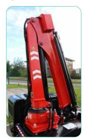
The Tracked Leveller 6.0 can be adapted with a crane kit that offers a maximum lifting capacity of 990kg with a max working radius of 4.3m.
