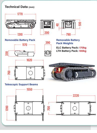
The four telescopic support beams on each corner provide added support for larger loads. The supports can extend the platform either longitudinally or laterally.
