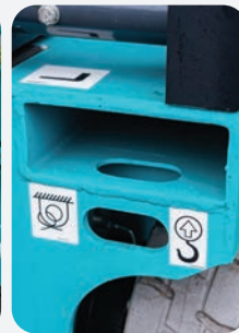
Lifting eyes are included for ease of transport or moving from level to level by crane.
