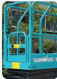
The SWSL14 comes fitted with a self-locking gate for operator safety
