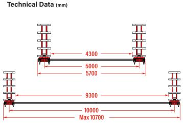
Please Note: Connecting Tube can be customised for any glass length between 1.7m - 12.0m.
