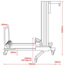
Note 1: Counterweights must be secured before lifting. Note 2: When using fork attachment the load must be centralised and secured.
