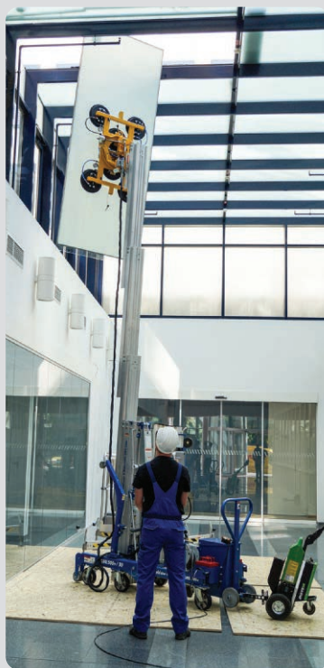
The GML500+ can also be used with its own optional glass vacuum lifter with radio remote for total control when glazing at height. The maximum capacity is reduced if using the VGL98 Glass Vacuum Lifter to 350kg.
