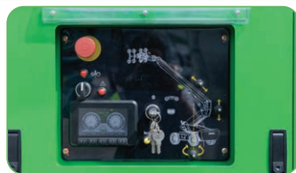
The control panel on the machine has a built-in display showing modes and capacities.
