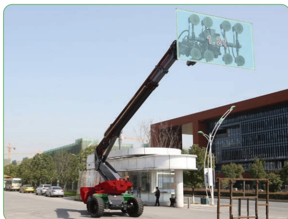
The Sky Robot 1500 has a maximum working radius of 13.95m and a maximum lifting height of 26.16m (capacity reduced)
