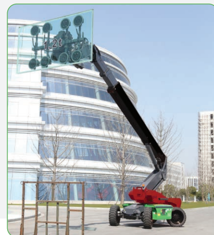
The Sky Robot 1500 is controlled by a high precision radio remote control
