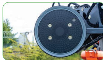
The Sky Robot 1500 comes with 8 black rubber vacuum pads to provide safe and reliable suction power.
